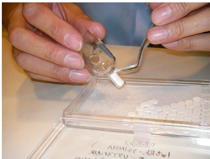
Fig. 4 Mount of disk sample into inner holder of sample cell
