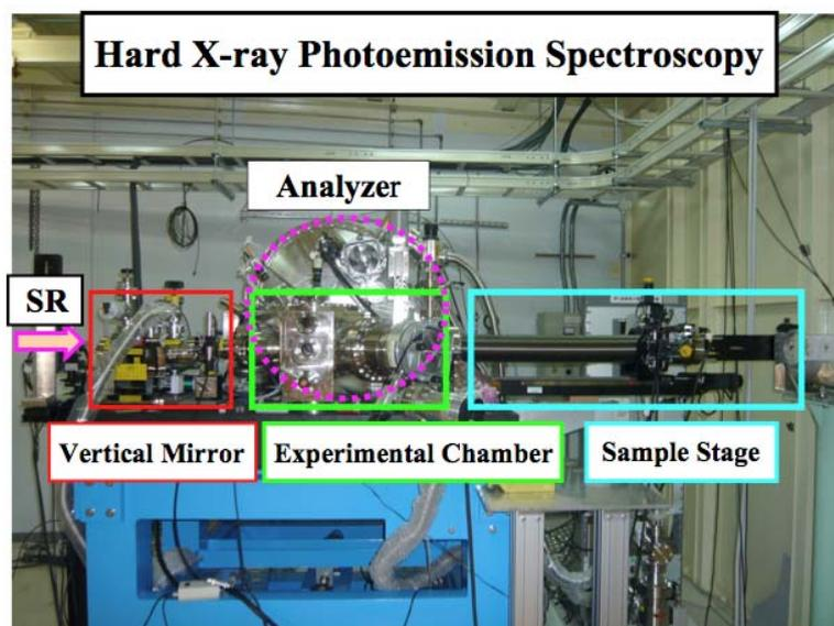
The aim of this course is to learn a principle of HAXPES and gain experience of measuring photoelectron spectra of various materials with 8 keV monochromated X-ray.
