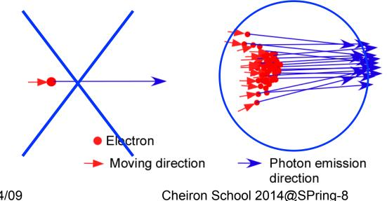
In the real world N electrons are distributed in a phase space, never degenerate on the same point. 1. Light source properties vs electron beam performance(6)
