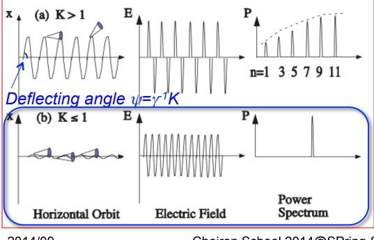
Spectral narrowing by resonant condition for a single electron is
